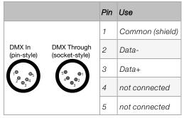
Up to 32 DMX Adapters (or other DMX devices) are allowed on a single control run. You must terminate the last device in the control run with a 120 ohm resister (connected between pins 2 and 3 (DMX- and DMX+) to prevent signal reflections or install a DMX Terminator Plug on the last device DMX through connector (see Accessories for ordering information).
