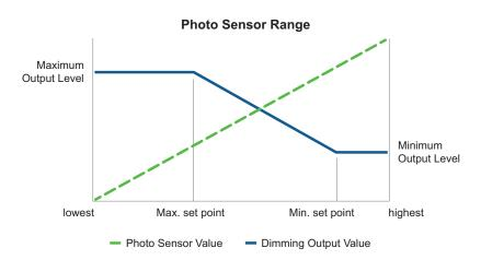
The rate that the dimming output changes is defined by the *open loop dimming rate* parameter which defines the time for dimming to go from lowest to highest or vice versa (default 65 seconds).
